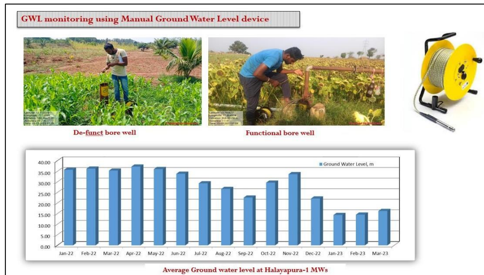
GWL monitoring using manual ground water level device and readings
