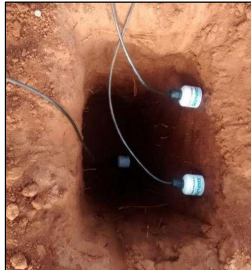
Schematic of HYDRA Probe Soil Moisture Sensor
