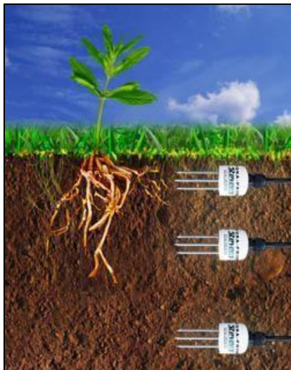
Schematic of HYDRA Probe Soil Moisture Sensor Measurement of Runoff
